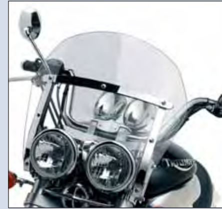
Summer Screen A9748040 Manufactured from Lexan Polycarbonate for additional strength and durability. Requires Front End Fixing Kit (A9738051)
