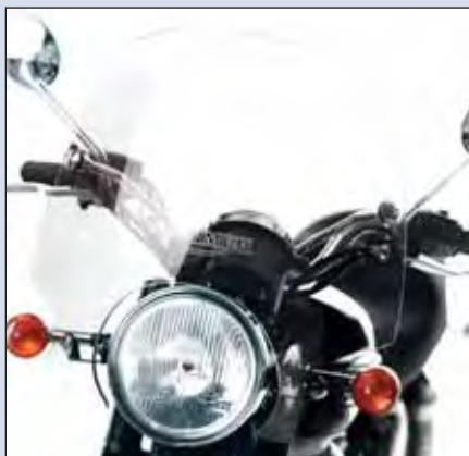
Summer Screen A9748029 Manufactured from Lexan Polycarbonate for additional strength and durability
